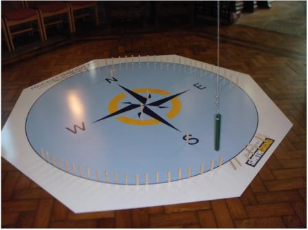
we hung a 2 kg sash weight on the bottom of the cable as a bob, securing it with three metal grips. The next task was to put in place the baseboard which had kindly been produced by Smith Signs Limited. This was a large octagonal design, with a compass rose showing the true north direction (the church being 17° off from an eastwest alignment), and really enhanced the presentation of the pendulum, as well as providing protection for the church floor.
